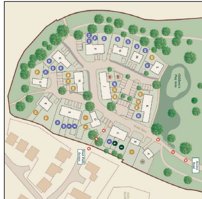
Layout of a development in Ticehurst showing pedestrian links and soft boundaries
